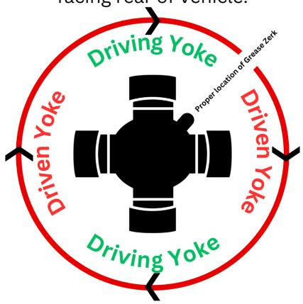
Greaseable U-Joints should be clocked to place the grease zerk under compressive load.
